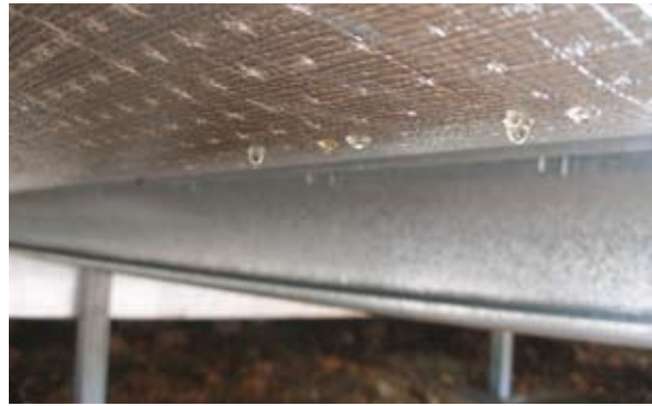
Demonstrating water permeability of Permifloor
