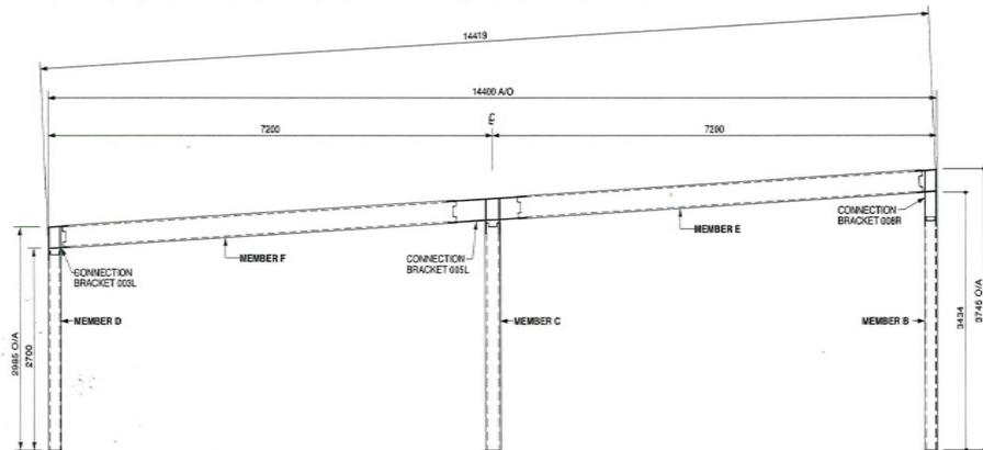
Fig.2 : Portal frame with hollow-flange Long Span Beam and connectors
