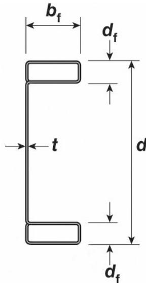
Fig.1 : Generic section of hollow-flange Long Span Beam
