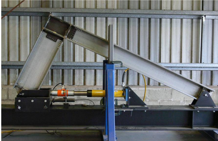
Fig.4 : Load testing of Long Span Beam portal frame knee connection
