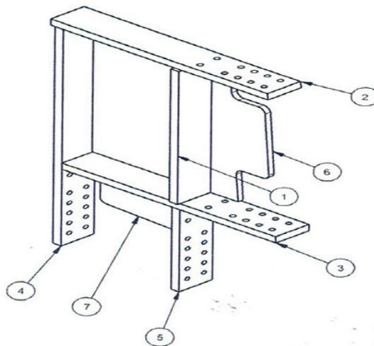
Fig.3 : Detail of hollow-flange Long Span Beam portal knee connector
