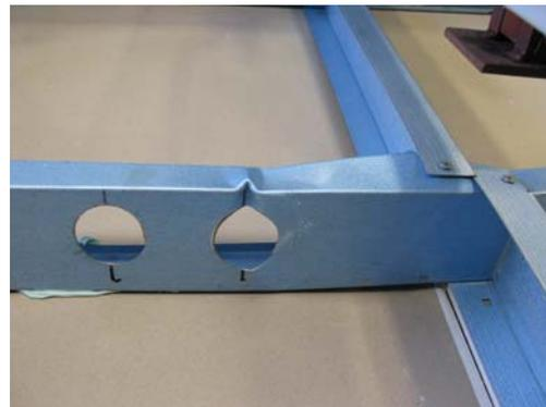
Figure 4. 90 x 0.55 mm Lipped Stud with pairs of 44 mm round holes, 400 mm Centreline Spacing – Failure.
