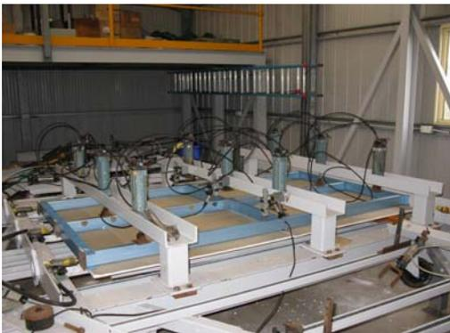
Figure 3. Test set up, 1.00 mm Lipped Stud with 38 mm round holes, 185 mm Centreline spacing.
