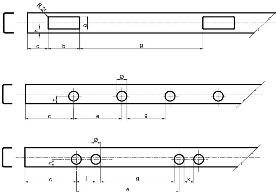
Figure 2. Hole configurations considered.
