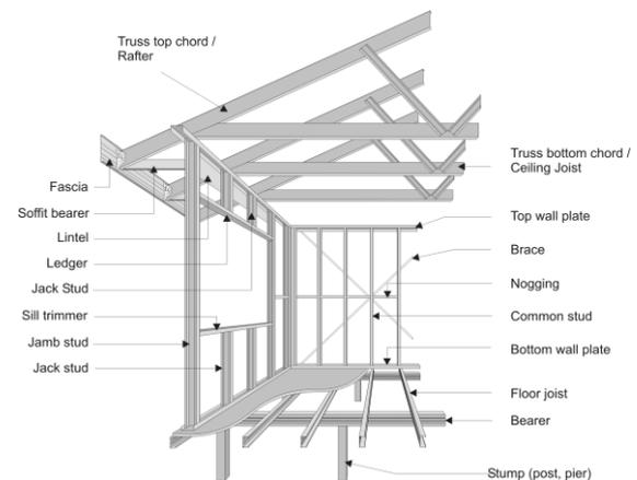
**Figure 2: Structural components of typical residential and low-rise structure [7]**
